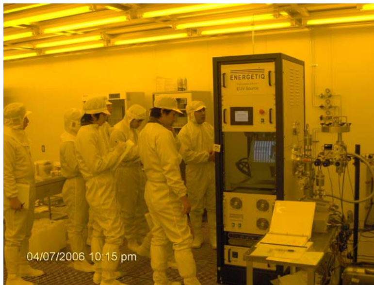
Figure 4: A simple flood exposure system
