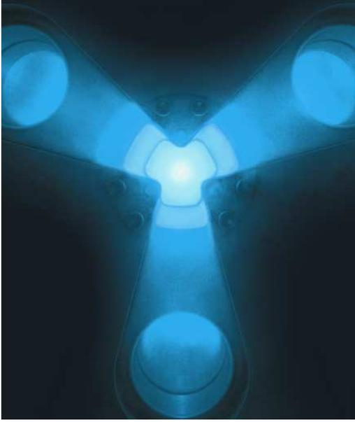
Figure 1: Visible light image of the EQ-10's three plasma loops.
