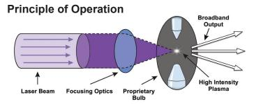
LDLS technology utilizes a laser to create an extremely small, high-brightness plasma with a broad spectral range.
